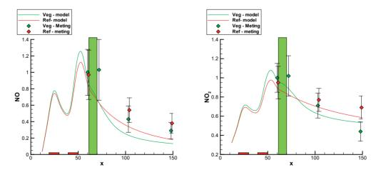
Figure 4. Normalised mean nitrogen oxides concentrations (NO left, NO<sub>2</sub> right) at 2 meters height. Green bar indicates the location of the vegetation, the red boxes the line sources. Green and red dots represent the ECN measurements, continuous lines: model results. Red: Along the reference measurement line, green: in front of and behind the vegetation barrier. Mean wind is blowing from the left.
