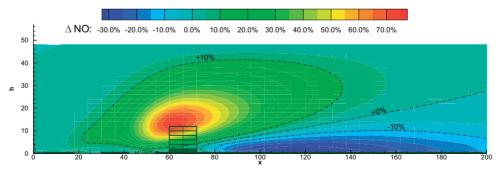
Figure 6. Mean relative difference in NO-concentrations with and without a vegetation barrier.
