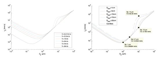
Figure 1. Deposition velocity as function of the particle size for different local wind speeds inside the vegetation canopy (leaf size = 0.15m, left) and different leaf sizes (wind speed =  $2 ms^{-1}$ , right).
