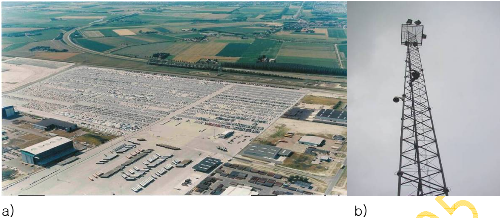
Figure 4: a) Location of the site (storage of 25.000 new cars) for which risk assessment is made; b) Detail of the on-site light tower for measurement of wind speed and wind direction.
