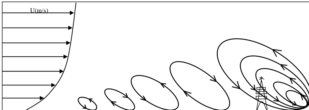
Figure 5. A superposed eddy model whose eddy size increases with downwind distance like dispersion of smoke, and the kinetic energy of the eddy decreases with the increase of eddy size because it is changed to heat energy. (neutral air)
