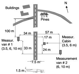
Figure 1. A schematic diagram of the measurement devices and their locations with respect to the road. The measurement heights are indicated in parentheses (Kukkonen et al., 2001).
