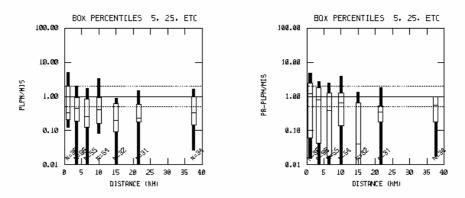
Figure 2. Residual analysis (Q=3) for PLPM and PR-PLPM, varying the distance from the source
