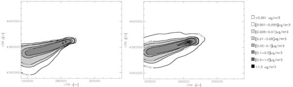
*Figure 4. PLPM (left) and PR-PLPM (right) estimated concentration at ground level. Triangle colour indicate measured concentrations at receptors positions. Kincaid, 31 5 1981, h 12.*
