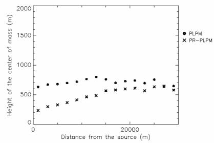
*Figure 1. Plume centre of mass height as a function of the distance from the source. Kincaid, 31 5 1981, h 13.*
