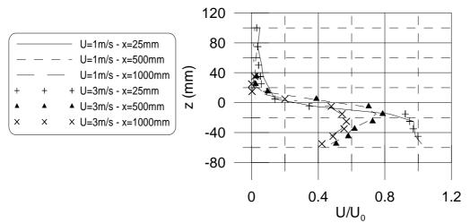
Figure 2. Velocity profiles showing independence of the ratio  $U_r/V$
