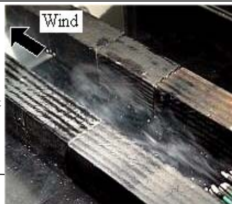
Figure 2. Flow for wind direction parallel to the street
