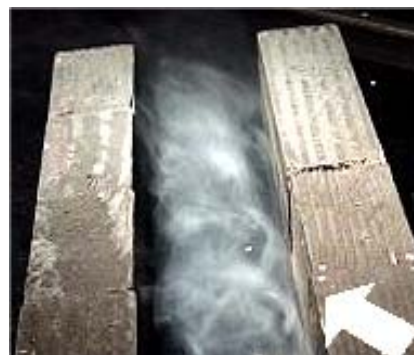
Figure 3. A spiral flow for wind direction oblique to the street ( \theta = 45^\circ )
