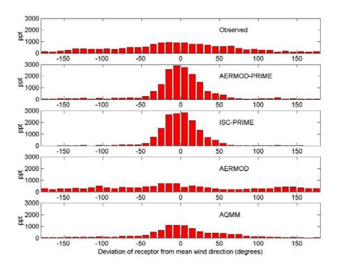
Figure 1. Concentrations as a function of the deviation of the wind direction from the line joining the centre of the source to the receptor.
