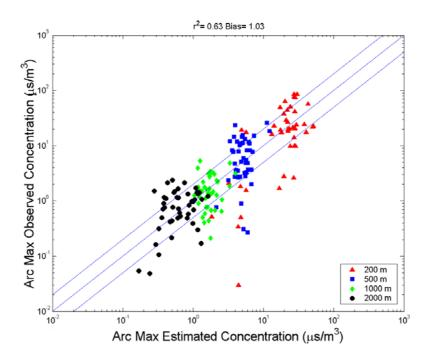
Figure 2. Comparison of arc maximum observed concentrations with estimates using Equation (1) in a Gaussian dispersion model.
