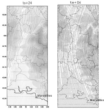
Figure 2. MM5 (on the left) and MINERVE (on the right) results. Flow streamlines at 10 m above the ground level. Time =  $t_0 + 24h$ . Topography is also represented.
