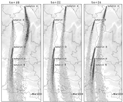
Figure 3. SPRAY results. Xenon activity concentration field. The concentration is averaged between 0 and 40 m. Times  $t_0 + 18h$ ,  $t_0 + 22h$ , and  $t_0 + 24h$ .
