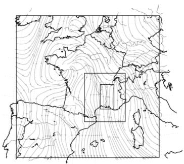
Figure 1. MM5 results. Three nested domains and the flow streamlines over the outer coarse domain, at 10 m above the ground level. Time =  $t_0 + 9h$ .
