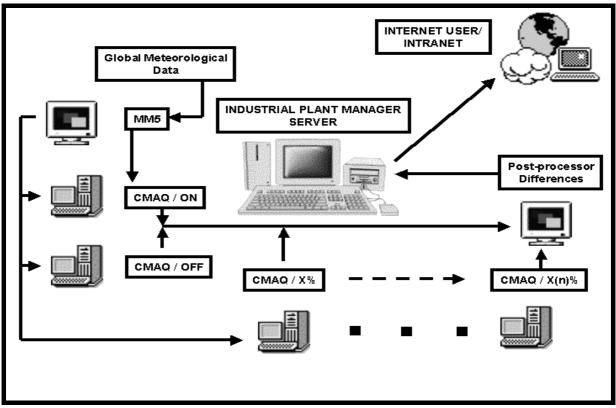
*Figure 2. Computer platform (TEAP) used to simulate different emission reduction scenarios for different large industrial plants.*
