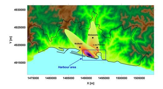
Figure 13. Test simulations with ADMS-Urban for the evaluation of the impact of harbour activities emissions on the urban area. Two cases are reported: one with SE wind of 5 ms<sup>-1</sup> intensity and one with S wind of 5 ms<sup>-1</sup> intensity. The pollutant simulated is NO<sub>x</sub> with arbitrary emission rates. The black line indicates the administrative boundaries of the city of Genoa, the blue rectangle indicates the most emissive harbour area.
