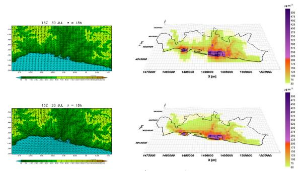
Figure 15. Results of the simulations for two summer days, July 30<sup>th</sup> (top) and July 20<sup>th</sup> (bottom). In the left column we report the maps with topography and 10 m wind fields obtained by the meteorological pre-processor for the afternoon time. In the right column we report the hourly mean concentration values at 2m above the ground level of NO<sub>x</sub> averaged on the whole day.
