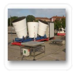
Figure 28. Rass/Sodar station with the Sonic Anemometer.
