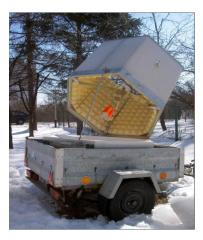
Figure 43. 1DDS SODAR antenna
