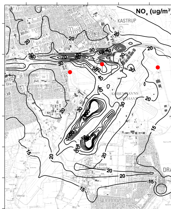
Figure 6. The average NO x concentrations for the year 2010. Maximum contour lines are 100 \mu\text{g m}^{-3} . Red dots are positions of monitors. Scale: 1 km between tick marks.
