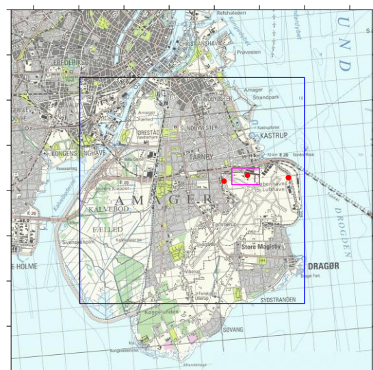
Figure 1. Map of the south-eastern part of Copenhagen where the airport is located. The blue square marks the OML domain of 10x10 km 2 and the red rectangle marks the MISKAM domain. Red dots are positions of measurements.
