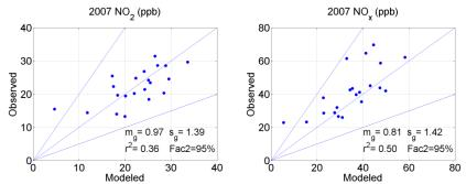
Figure 4. Comparison of modeled and measured annually averaged NO2 and NOx concentrations at 21 sites in the SoCAB.
