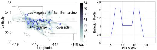
Figure 1.Gridded NO<sub>x</sub> emissions and monitoring stations located in the South Coast Air Basin, Los Angeles. The right panel shows the assumed temporal profile of NO<sub>x</sub> emissions.
