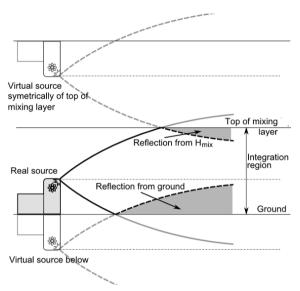
Figure 2. Chart of straight-line Gaussian solution with reflections.
