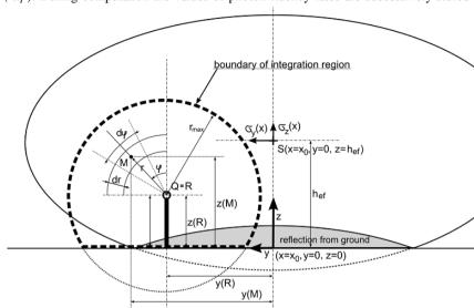
means the number of receptors being simultaneously taking into account,  $I_{total}$  stands for total number of the 10-meter segments of the plume separation (so far selected value  $I_{total}=720$ ). Total fluency rates, total fluency and corresponding total cloudshine doses/dose rates are generated by summing up the values in particular time steps.
