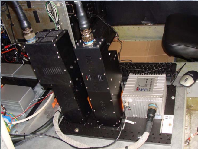
Hyspex sensor and inertial platform
