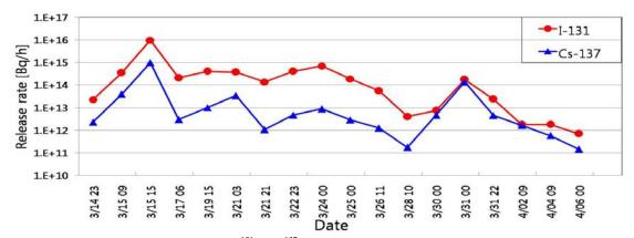
Figure 1. Time series of the source term for  $^{131}\mathrm{I}$  and  $^{137}\mathrm{Cs.}$
