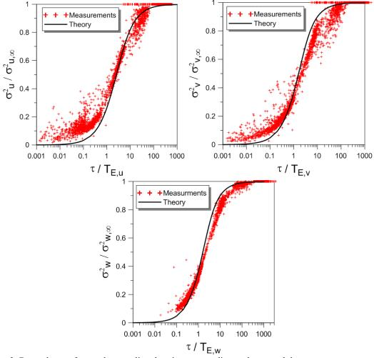
Figure 2: Dependence of  $\sigma_i$  on the sampling duration  $\tau$ , according to theory and the measurements.
