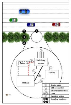
Figure 1: Schematic diagram of the sampling site showing the sampling points and experiment setups as described in the text. Please note that the figure is not in scale.
