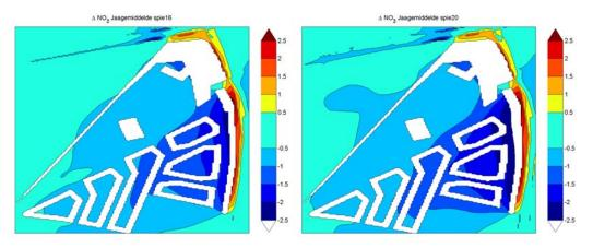
Figure 5 : Resulting effect of the building wall on the yearly average NO<sub>2</sub> concentrations for two different wall heights (left: 16 m high buildings, right: 20m high buildings). Scale is concentration difference in  $\mu$ g/m<sup>3</sup>.
