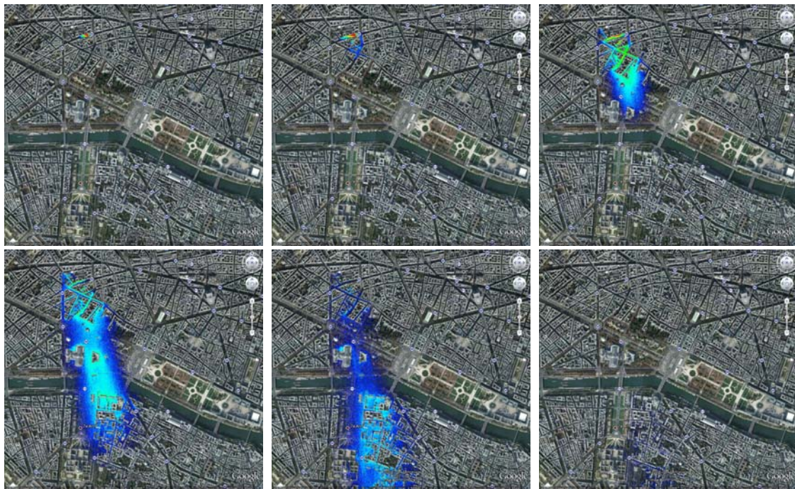
Figure 5. Radionuclide activity concentration (in \text{Bq}\cdot\text{m}^{-3} ) near the ground at six instants after the explosion.
