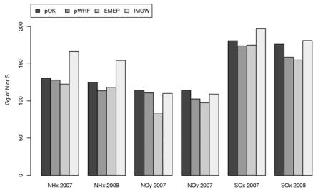
Fig. 3 National deposition budget for  $NH_x$ ,  $NO_y$  and  $SO_x$  modelled with FRAME, EMEP and provided by spatial interpolation approach used by IMGW.
