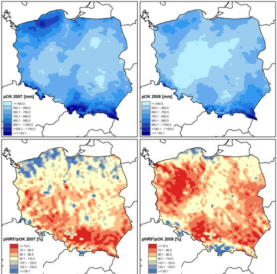
Fig. 1 Interpolated precipitation (top row) and relative differences between the WRF and interpolated rainfall (bottom) for years 2007-2008
