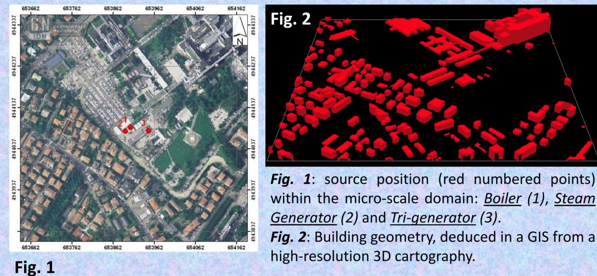
Emission sources: The plant was sized according to safety criteria and the tri-generation unit is supported by two auxiliary devices: one conventional boiler and one steam generator, which emission patterns vary according to the hourly average fuel consumption in the monthly mean day. Stack heights are all equal to 10 m, except for the tri-generation unit (15 m).
