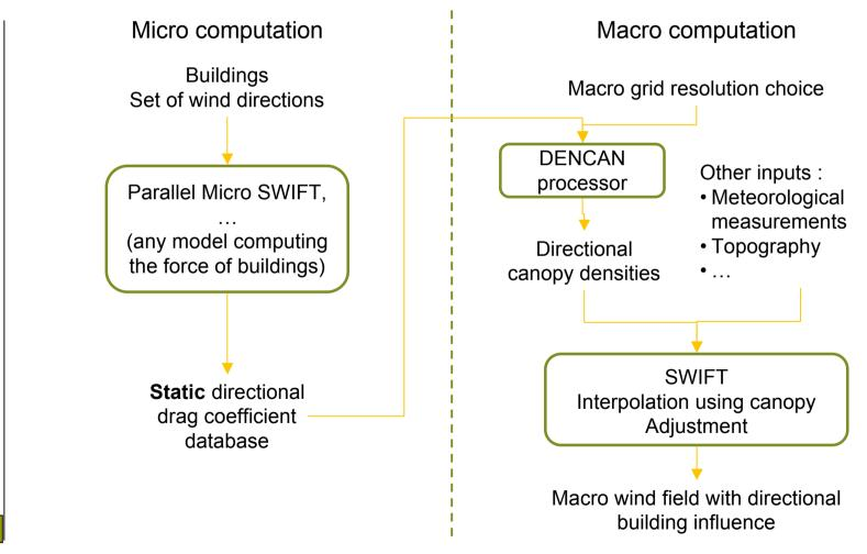
Drag coefficients are computed using a local scale code, for instance Micro SWIFT, for a set of wind directions and stored in a static database
