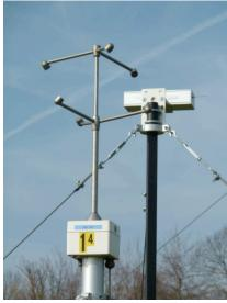
Ultrasonic anemometers (front) and PID (behind)
