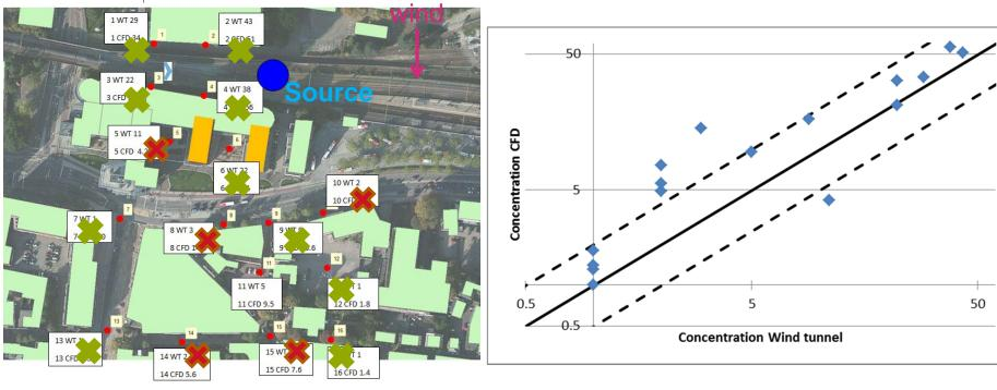
11 measurements (out of 16) are within a factor of 2 Plume width and upwind dispersion are calculated correctly
