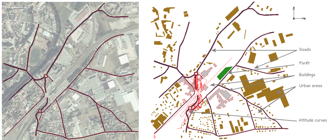
Figure 2. Aerial view of domain with roads (left) – numerical model of terrain (right)
