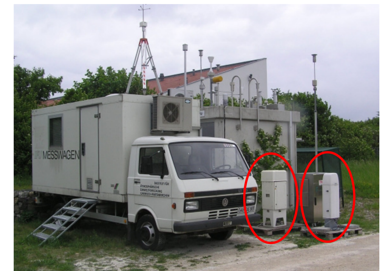
Ceilometers at the site in Augsburg. The right one is the instrument used for the continuous measurements
