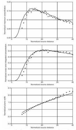
Fig.1 Comparison between results from wind tunnel (diamonds) and AUSTAL2000 (solid line)
