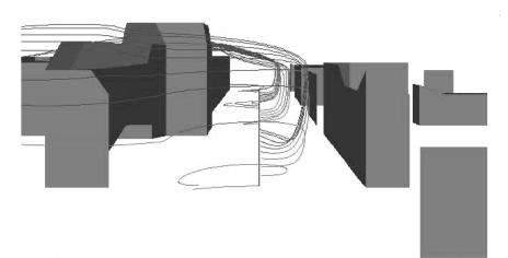
Figure 3. Simulation of a tracer experiment in an urban street canyon with MITRAS. Buildings are indicated as shaded blocks. The tracer is released at a line source in the centre of the street. Advection of the tracer is visualised by streamlines. Above the urban canopy, the wind is blowing from right to left (Schluenzen, 2002).
