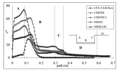
Figure 4. Comparison of the normalised concentration  $c^*$  along the path ABCD for the cavity with W/H=2 (A and C correspond to 75% of the cavity depth, while B and D are equal to its width) after Sahm et al. (2001).
