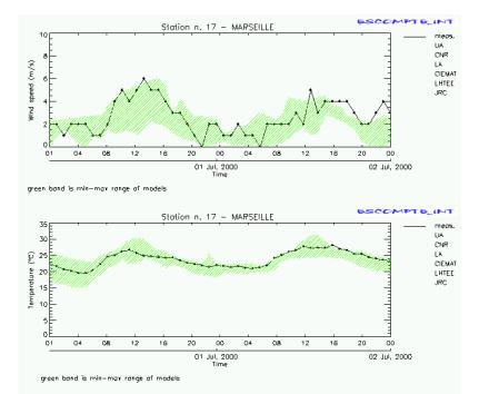
Figure 5. Range of wind speed and temperature in Marseille on 1 July 2000 resulting from simulations with six different urban scale models compared to corresponding results of the ESCOMPTE pre-campaign (cf. http://rem.jrc.cec.eu.int/escompte int/RESULTS/).
