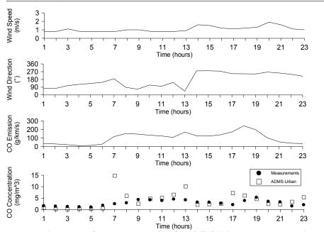
*Figure 4. Comparison between measured and modelled CO concentrations on 27 November 2001. The corresponding wind and emission input data have been reported above.*
