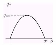
Figure 2. Fundamental traffic diagram.
