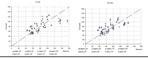
Figure 2. Scatter plots of observed versus modeled ozone peak concentrations at various percentiles
