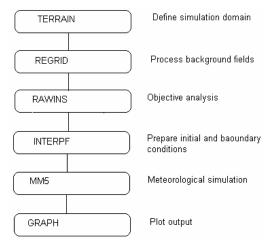
Figure 1. Flow chart of MM5 modeling system.
