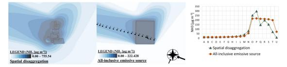
Figure 2. Ammonia concentration maps for different spatial disaggregation of emissive source areas.
