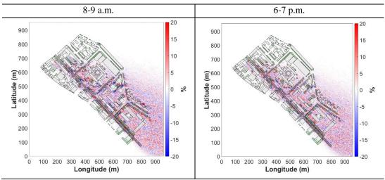
**Figure 2.** Spatial distribution of the relative difference (in percentage) between the CAV scenario and baseline case across the computational domain, for 1.5 m high horizontal streamlines. Contours refer to the period of 8-9 a.m. (with a wind velocity of 1.9 m·s<sup>-1</sup> and a wind direction of 289°), and 6-7 p.m. (with a wind velocity of 3.7 m·s<sup>-1</sup> and a wind direction of 293°).
