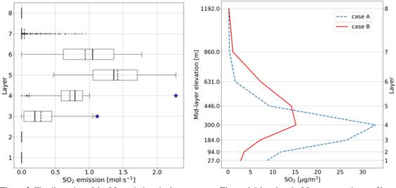
**Figure 3.** The dispersion of the SO<sub>2</sub> emissions in the individual layers with the plume rise. The stars represent position and magnitude of the emission sources without the plume rise. The bold line within the box is a median and the dashed line is an average.
