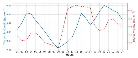
**Figure 7.** Mean daily profiles of SO<sub>2</sub> concentration difference without and with the plume rise for the whole domain - blue line (29x33 grid cells, first 8 vertical layers) and source vicinity - red dashed line (5x5 grid cells, first 8 vertical layers).
