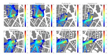
FIGURE – Predictions *vs.* Ground Truth (PMSS simulations) : integrated concentration fields (over 2 hours) in Paris (log scale)
