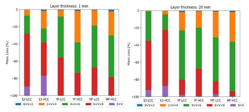
The figures show, in percentage, the mass loss (in relation to the initial mass) within the five different velocity groups, for all species. The increasing ash layer thickness results in greater ash mass losses at lower wind velocities.
