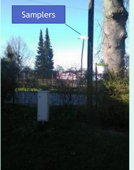
Figure 1. Passive samplers (under the white cover) at measurement site.
