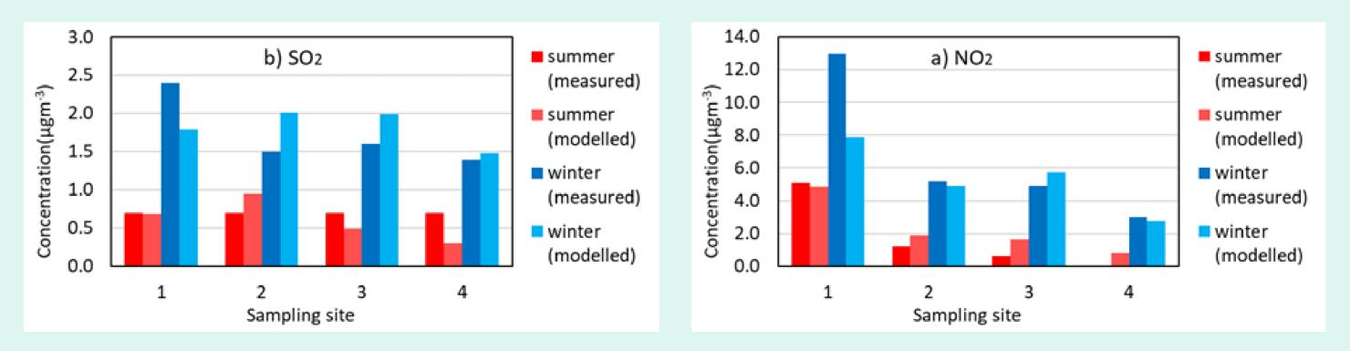
**Figure 4.** Measured winter- and summertime concentrations of  $NO_2$  and  $SO_2$  in sampling sites compared to model results
