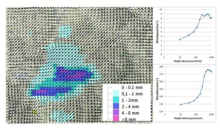
**Figure 4.** Meteorological data (COSMO-DE) for the realistic scenario (third hour): wind field (height 73 m) and precipitation (left). The plant is marked with a yellow dot. The right side shows the vertical profile for wind velocity and wind direction at the plant site up to 1000 m over ground level.
