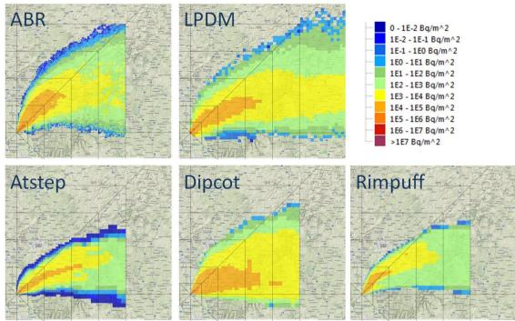
Figure 5. Total Deposition of I-131 for the models ABR, LPDM, Atstep. Dipcot and Rimpuff.
