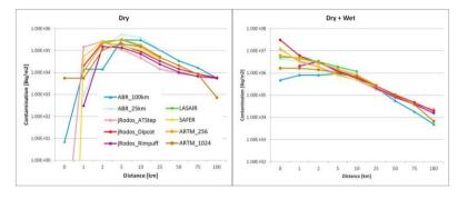
Figure 2. Deposition of Iodine 131 in  $Bq/m^2$  for neutral conditions: Dry deposition (left) and washout (right). Here, a homogeneous precipitation rate of 2 mm/h has been assumed.
