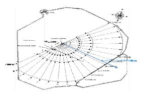
Figure 1: The whole measurement area in CEA-CESTA for the ammonia experimental test cases; sensor arcs locations (distances from the release system :  $20 \, \text{m}$ ,  $50 \, \text{m}$ ,  $100 \, \text{m}$ ,  $200 \, \text{m}$ ,  $500 \, \text{m}$ ,  $800 \, \text{m}$  and  $1700 \, \text{m}$  for corresponding referenced letters A, B, C, D, E, F, G)
