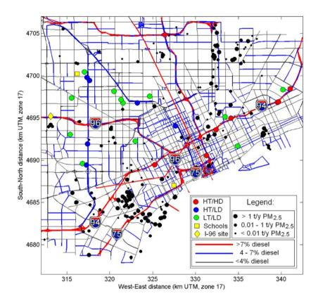
**Figure 1.** Modeling domain for the NEXUS study. Major highways are shown as red and blue lines (for > 7% diesel and 4-7% diesel fraction) and other roads – as black lines. Model receptors are shown in red, blue and green circles for the HD, LD and LT traffic exposure group, respectively. Stationary sources are shown as black dots (symbol size indicates the magnitude of PM<sub>2.5</sub> annual emissions).
