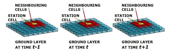
Figure 2. Examination of air-pollution concentrations in neighbouring cells to estimate model error in time and space
