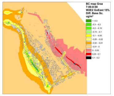
Figure 3: Example of a black carbon concentration difference map for Graz. Results of the ITS scenario and the base scenario have been averaged over all meteo conditions. Buildings in grey, units: μg/m<sup>3</sup>.
