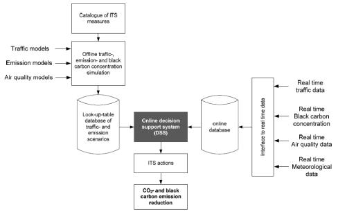
Figure 1. The CARBOTRAF system
