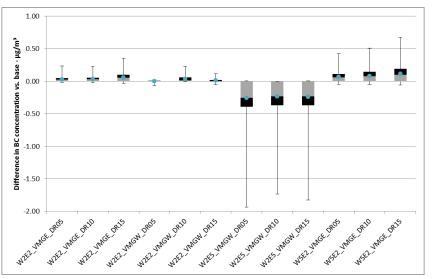
Figure 5. Boxplot of the difference in BC concentration vs. the base scenario, per ITS scenario, for BC monitor location 1, western arterial, Graz. Boundary condition 7:00 – 8:00, units μg/m<sup>3</sup>.
