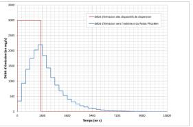
**Figure 4.** Yperite rate release (in mg.s<sup>-1</sup>) within the dispersal device and to the atmospheric environment.
