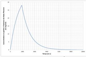
**Figure 3.** Yperite concentration (in mg.m<sup>-3</sup>) evolution inside the exhibition hall.
