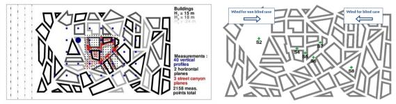
Figure 1. Computational domain with buildings, wind velocity measurement positions and sources positions.
