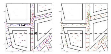
As seen before, TKE is overestimated at roofs' height so that a larger as expected part of the plume, rising up the street canyon, moves inside the enclosed courtyard upwind, where PMSS code overestimates concentration, as shown in figure 4.
