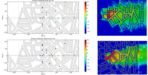
Figure 4. Concentration field at a height of 7.5 m and relative errors compared to observations for continuous release from source S5 (PMSS at the top and Code\_SATURNE at the bottom).
