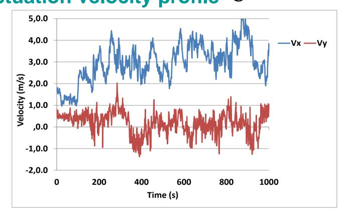
Measurements on the meteorological mast (vane anemometers, weather-cock) : two velocity components (1 Hz)
