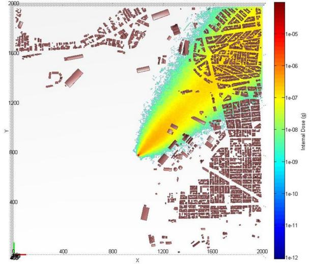
**Figure 16.** Horizontal distribution of the contaminant's total internal dose at the height of 1.3 m (time = 1000 s) produced by the QUIC-Plume model at Keratsini port.
