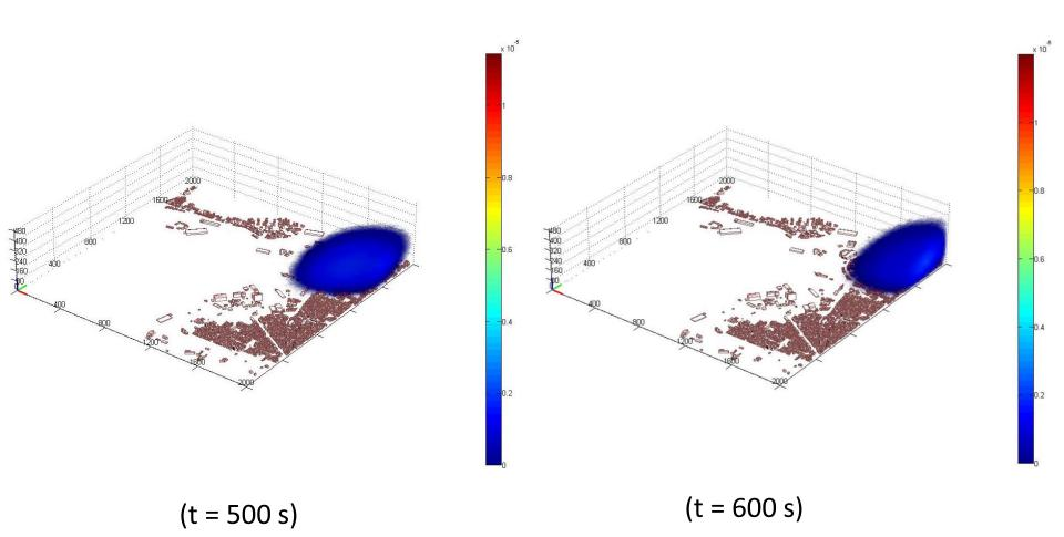
**Figure 11.** Illustration of the temporal evolution of the contaminant's plume produced by 3D simulations of the QUIC-Plume model at Keratsini port (in  $g/m^3$ ).
