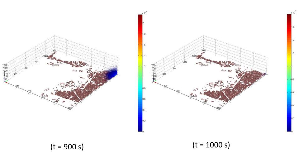
**Figure 13.** Illustration of the temporal evolution of the contaminant's plume produced by 3D simulations of the QUIC-Plume model at Keratsini port (in  $g/m^3$ ).
