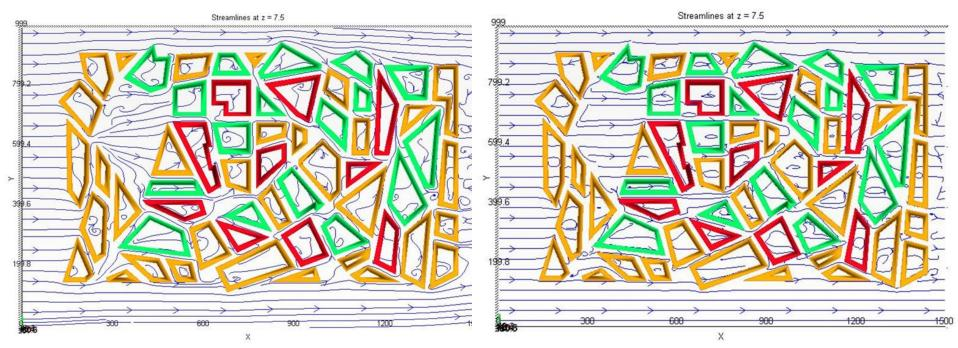
**Figure 1.a.** Horizontal streamlines at 7.5 m extracted by QUIC-CFD model
