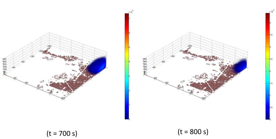
**Figure 12.** Illustration of the temporal evolution of the contaminant's plume produced by 3D simulations of the QUIC-Plume model at Keratsini port (in  $g/m^3$ ).
