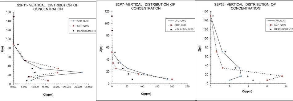
**Figure 4.** Comparison of concentration's vertical distribution for S2 source, extracted from the two models' simulations separately with measurements at 3 different points.
