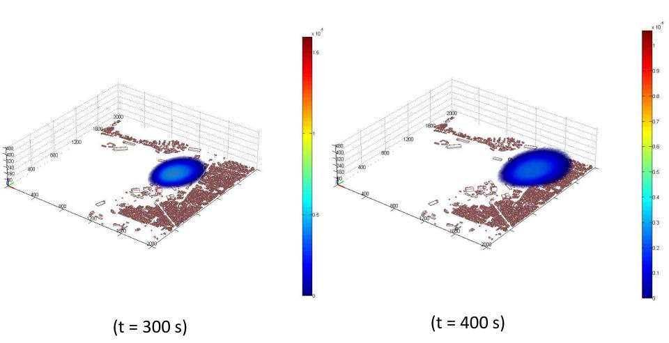
**Figure 10.** Illustration of the temporal evolution of the contaminant's plume produced by 3D simulations of the QUIC-Plume model at Keratsini port (in  $g/m^3$ ).
