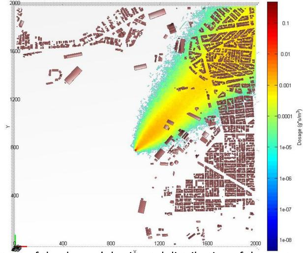
**Figure 14.** Contour of the dosage's horižontal distribution of the contaminant at the height of 1.3 m (time = 1000 s) produced by the QUIC-Plume model at Keratsini port.
