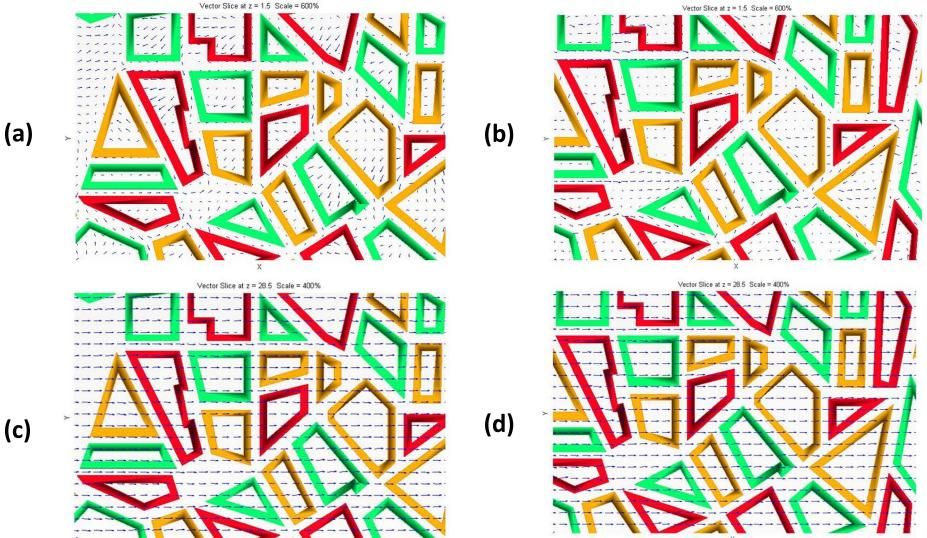
**Figure 2.** Wind field in the small domain at the levels of 1.5m and 28.5m extracted by the QUIC-CFD (a and c) and QUIC-URB (b and d) codes.
