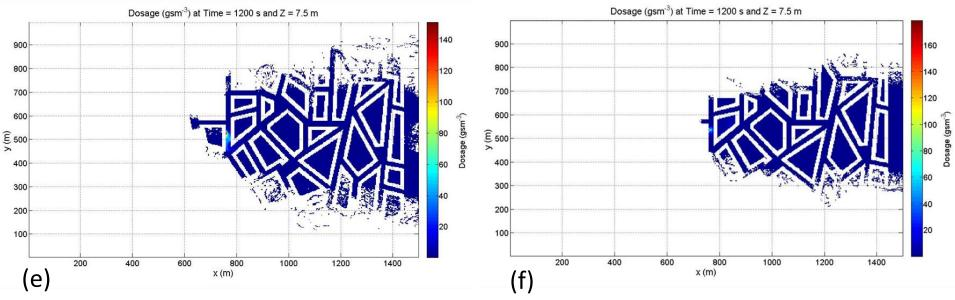
**Figure 6**. Simulations with QUIC-CFD model are illustrated on (a), (c) and (e) pictures for S2, S4 and S5 sources respectively. Simulations with QUIC-URB model are illustrated on (b), (d) and (f) pictures for S2, S4 and S5 sources respectively.
