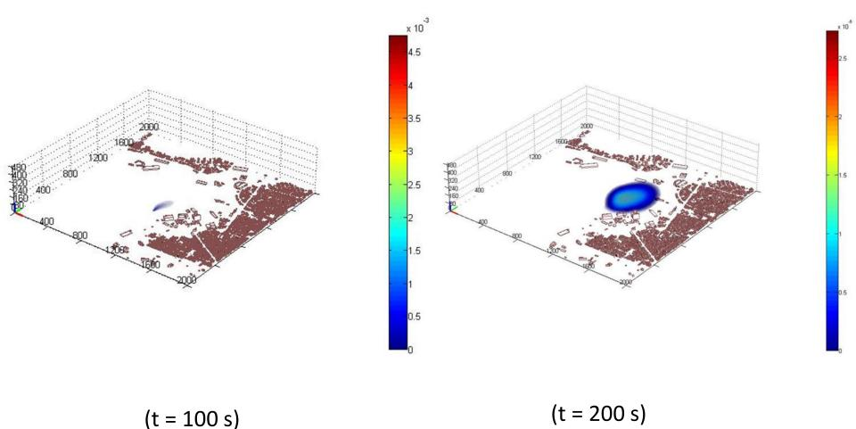
**Figure 9.** Illustration of the temporal evolution of the contaminant's plume produced by 3D simulations of the QUIC-Plume model at Keratsini port (in  $g/m^3$ ).
