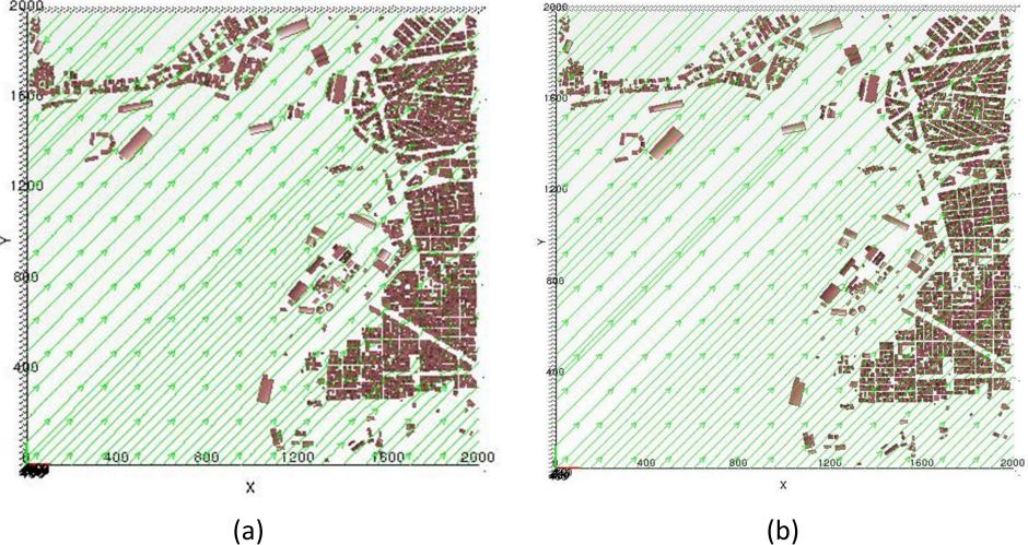
**Figure 8.** Depiction of the wind flow pattern at the height of 3 m (a) and 15 m (b) at Keratsini port with streamlines produced by QUIC-URB simulations.
